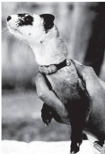
Figure 3. Capsules with high power output (Telonics, Inc., Mesa, Ariz.) (version B-1 of table 1) were attached to harnesses and tested on surrogate prairie dogs ( Cynomys spp.) in 1982. Photograph by D. Biggins.
