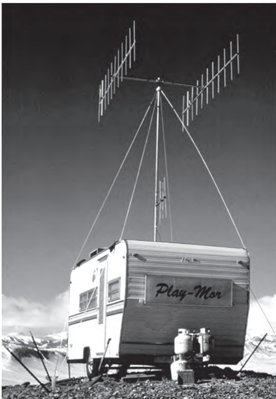
Figure 13. Camper trailer fitted with rotatable, 11-element, dual-beam Yagi array, used to radio track black-footed ferrets ( Mustela nigripes ) at the Meeteetse, Wyo., study area in 1983–84. Photograph by D. Biggins.
