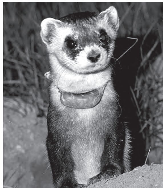
Figure 8. A 13-g transmitter package (version D-1 of table 1) from Wildlife Materials, Inc. (Murphysboro, Ill.), with Teflon tubing covering most of the acrylic potting material (used on black-footed ferrets [ Mustela nigripes ] during 1984). Photograph by D. Biggins.
