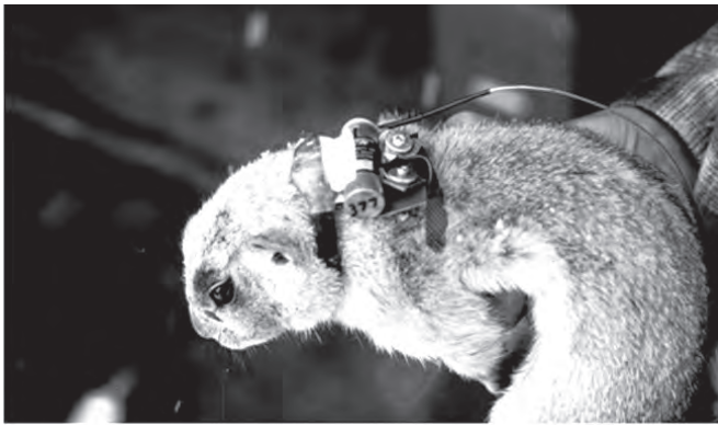
Figure 3. Capsules with high power output (Telonics, Inc., Mesa, Ariz.) (version B-1 of table 1) were attached to harnesses and tested on surrogate prairie dogs ( Cynomys spp.) in 1982. Photograph by D. Biggins.
