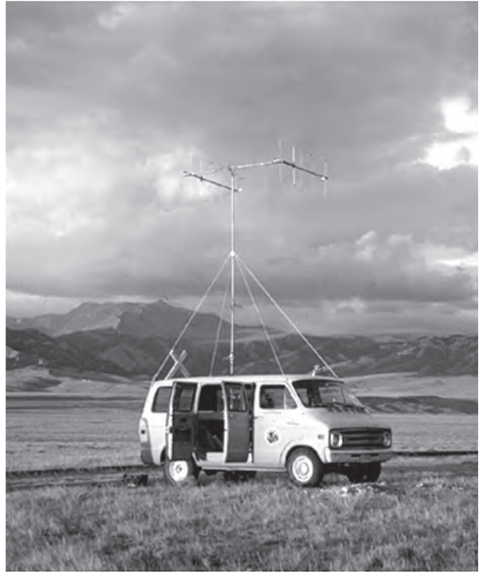
Figure 14. Truck-mounted, collapsible, 5-element Yagi array used to radio track black-footed ferrets ( Mustela nigripes ) at Meeteetse, Wyo., during 1982–84. Photograph by D. Biggins.
