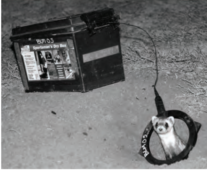
Figure 3. Automated passive integrated transponder readers in waterproof boxes may be left at burrows occupied by black-footed ferrets ( Mustela nigripes ). Transponder numbers will be recorded as the ferret passes near (or through) the loop antenna placed to encircle the burrow entrance.
